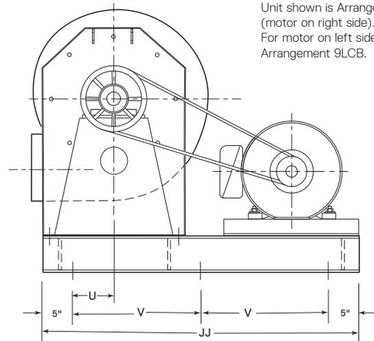
Unit shown is Arrangement 9RCB (motor on right side). For motor on left side, specify Arrangement 9LCB.
