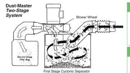
First stage cyclonic separator filters large dust and particles into container. Smaller particles pass through blower wheel into second stage bag.
