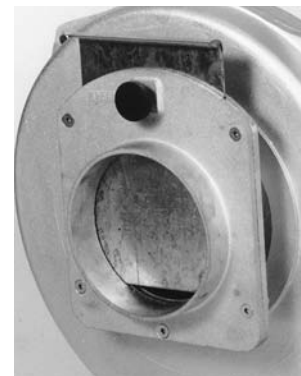
SLIDE GATE DAMPER Available for 4, 5, 6, 7, 8 and 10 inch inlets or outlets. Cast aluminum frame, galvanized steel gate. Suitable for duct work. Dimensions on page 21. Add inlet/outlet guard if not ducted. Not available on downblast discharge position.
