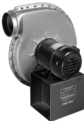
PB-14 with continuous flange added to ensure meeting "low leakage" requirement in evacuating oil mist at 14" SP WG on discharge.
